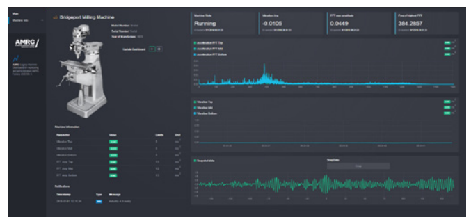
Figure 9: Website dashboards developed to visualise data collected for the Bridgeport Turret mill. Top: General overview; Bottom left: High frequency, detailed current analysis; Bottom right: High frequency, detailed vibration analysis.
