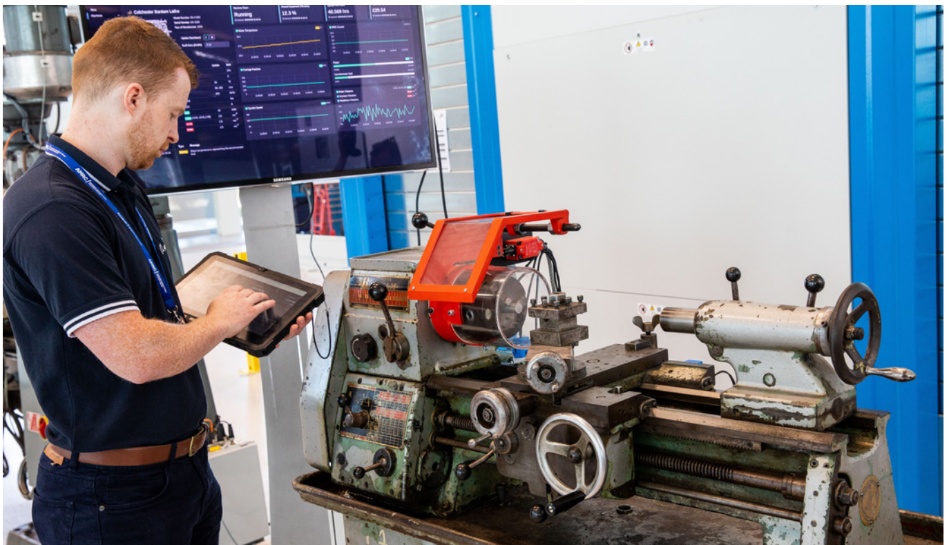
Figure 1: A 1956 Colchester Bantam lathe retro-fitted with ultra-low cost sensing equipment attached.
