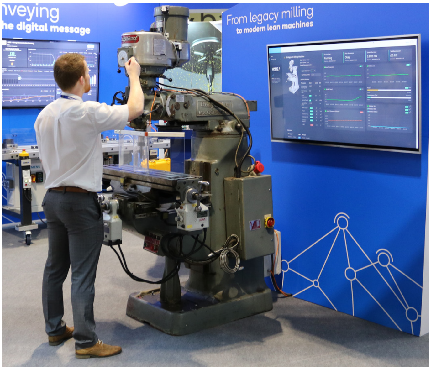
Figure 6: A 1980’s Bridgeport Turret mill with high fidelity sensor equipment attached.
