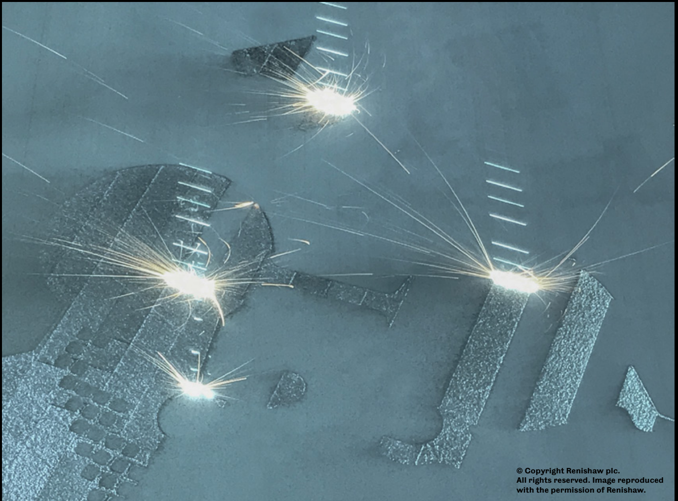
Renishaw RenAM500Q multi laser system melting metal powder.
