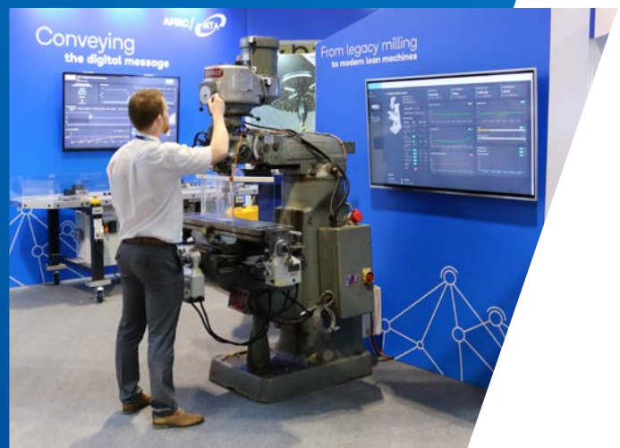
Demonstrating the legacy milling machine retrofitted with low cost sensors.
