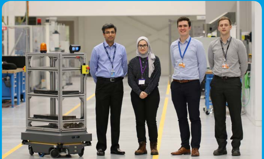
MiR200 with racking, integrated flashing beacon and direction indicator projector. (Left to right) Amer Liaqat and Sema Al-Attbi of Airbus UK; Dr Lloyd Tinkler and Dr Scott Dufferwiel of the AMRC.
