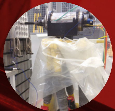
The legs of a hexapod robot offer a greater degree of manoeuvrability when machining large components
