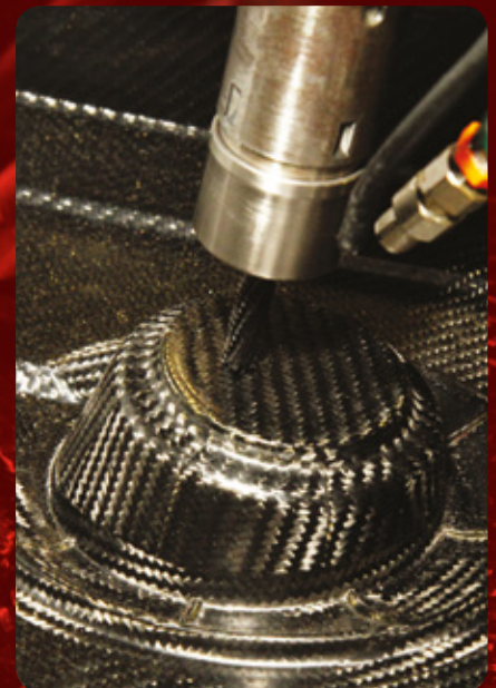
Milling carbon fibre reinforced plastic
