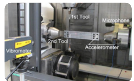
Parallel machining setup at the AMRC
