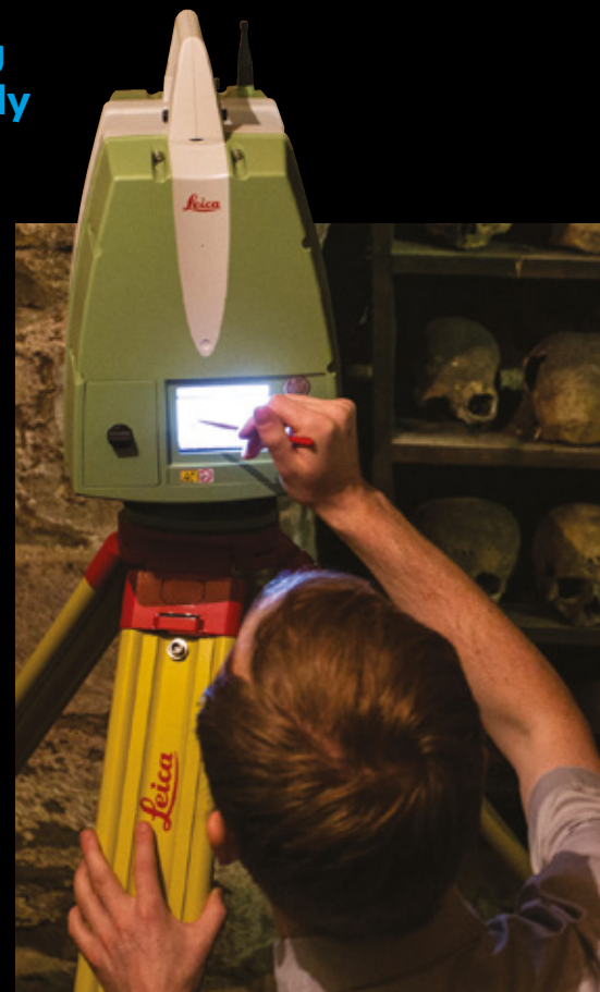
Tom Hodgson operating the Leica ScanStation P20 laser radar inside the Rothwell Holy Trinity Church Ossuary.
