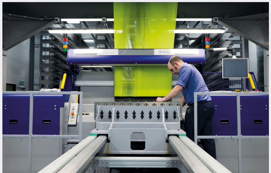
AMRC technical fellow, Steffan Lea processing silicon carbide fibre on a 3D weaving loom.
