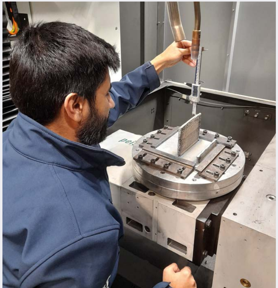
Muhammad Shamir, technical lead within the AM team at AMRC North West, measuring height of the wire arc additive manufactured (WAAM) wall to control layer height and process parameters.
