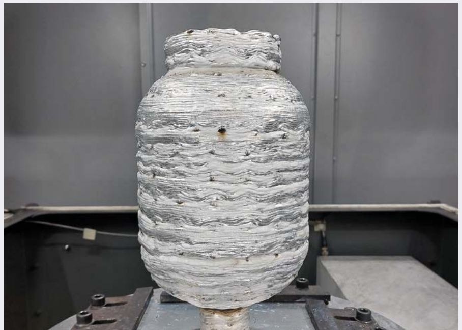
Showing the tank after it has been manufactured using wire + arc additive manufacturing.
