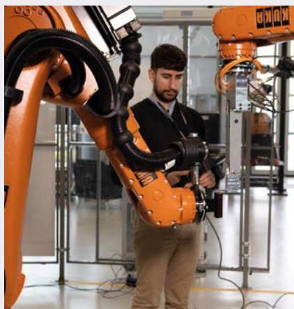
AMRC technical lead for novel robotics, Gianmarco Pisanelli, demonstrating robotic coil winding technique.
