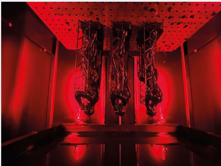
The three miniature replicas being 3D-printed using the Photocentric LC Magna 3D Printer.
