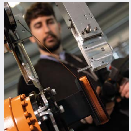
AMRC technical lead for novel robotics, Gianmarco Pisanelli, demonstrating robotic coil winding technique.
