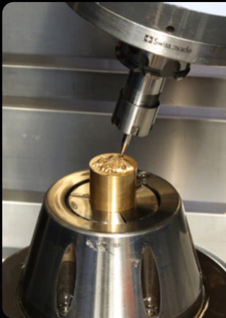
The portrait being micro-machined into brass using the Starrag Bumotec machine.
