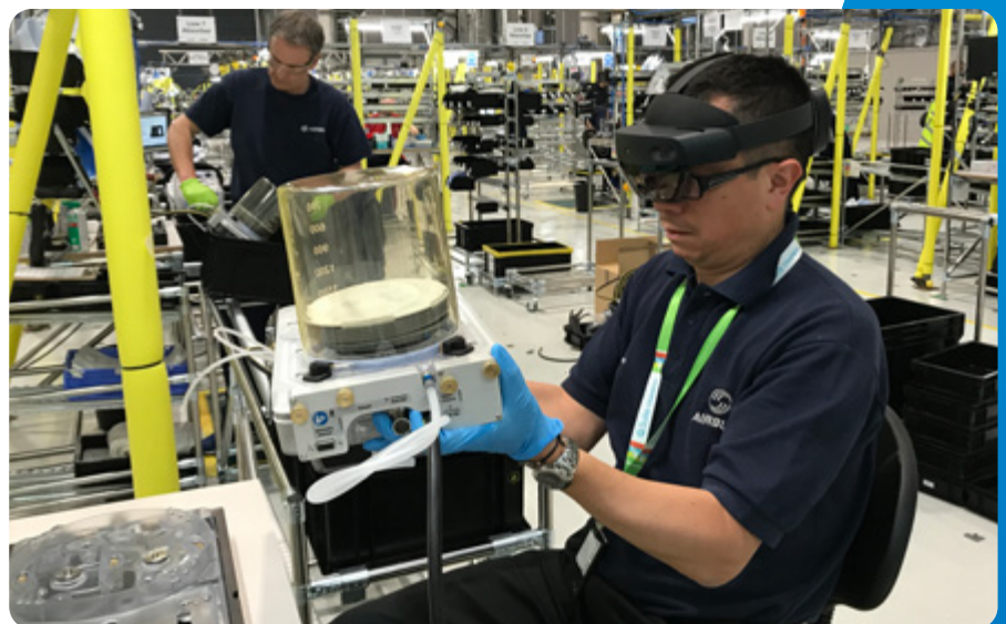
Airbus employees using the Microsoft HoloLens kits on ventilator production lines set up at AMRC Cymru.
