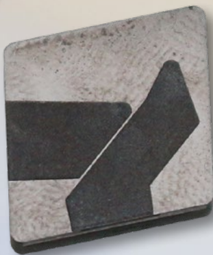
A low cost cutting tool with an embedded sensor.
