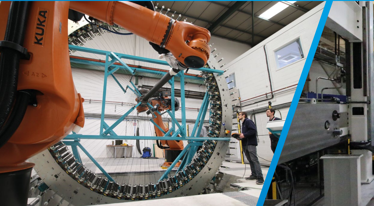
New tech: The radial braider, left, and other market leading equipment installed by the AMRC to manufacture preforms and develop enabling technology for commercialisation including joining, automation and impregnation.
