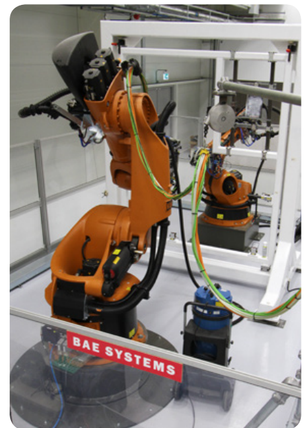
The robotic countersinking cell at the AMRC Factory 2050.
