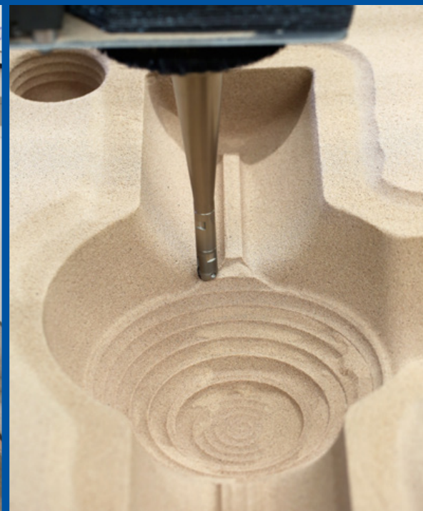
A sand mould being machined from a block of bonded sand.
