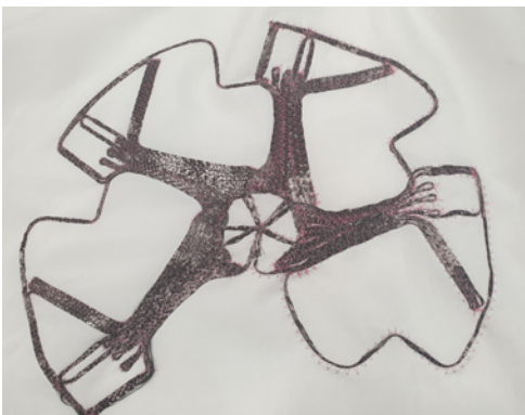
Fibre placement in all orientation
