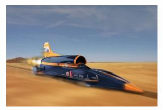
The Bloodhound car is powered by a Eurojet EJ200 engine, as used in the Eurofighter Typhoon aircraft, plus a Falcon hybrid rocket. A Cosworth CA 2010 Formula 1 motor pumps fuel to the rocket and provides power to the car's electrical and hydraulic systems. The car's body, chassis and control systems will meanwhile rely on a range of advanced design and manufacturing techniques.
