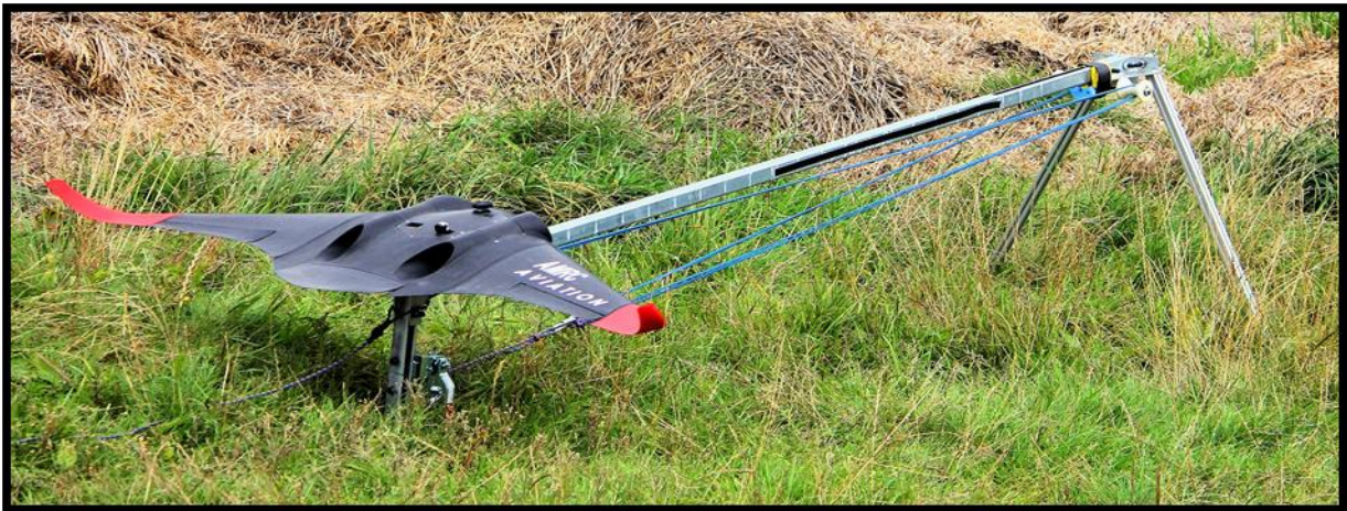
UAV ready for launch on catapult.
