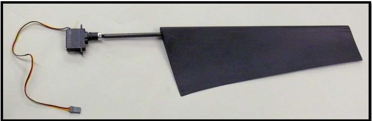
Starboard elevon with servo, adapter and torque tube.
