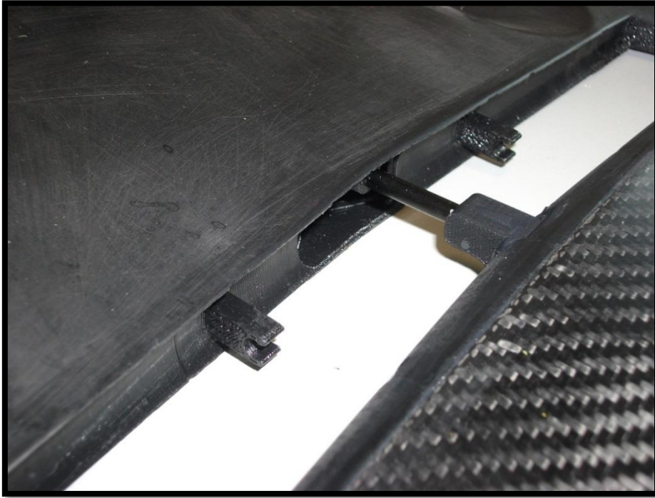
Duck-tail attachment points and lever.
