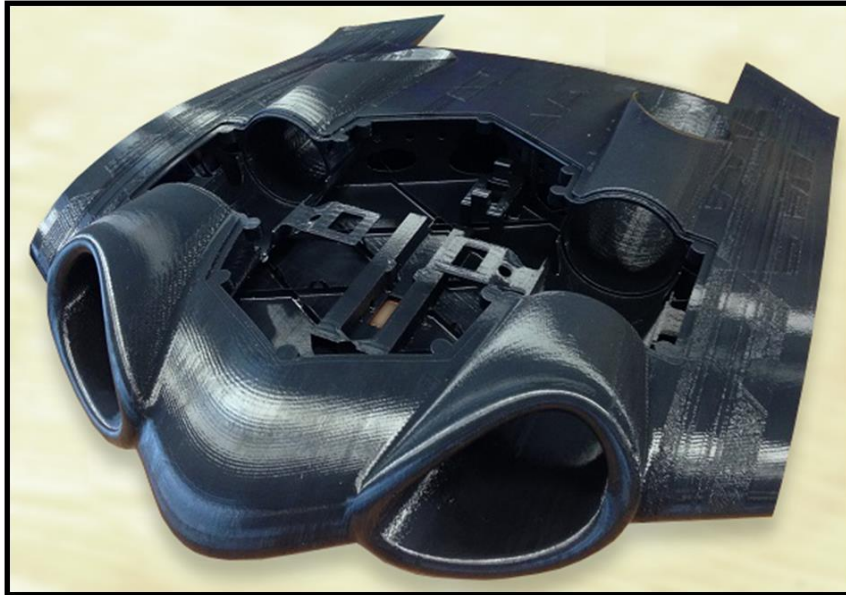
FDM printed one-piece centre body.
