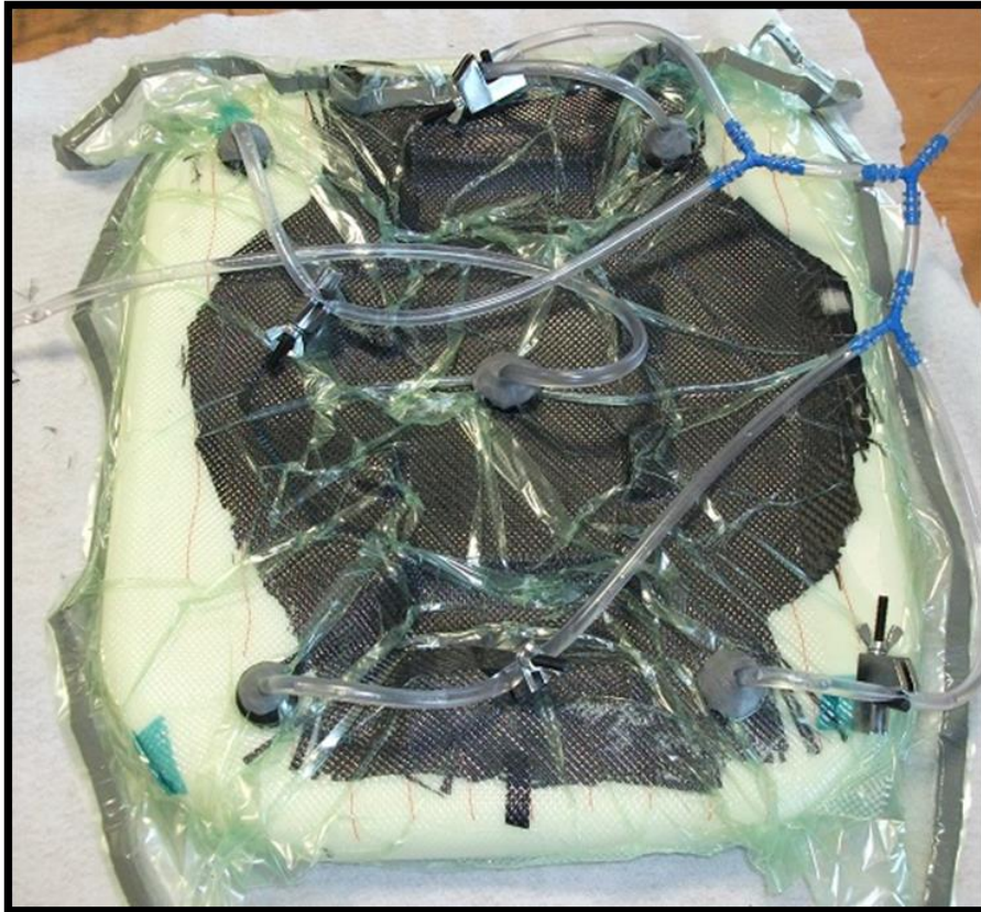
Vacuum infusion of the top hatch using an FDM printed mould.
