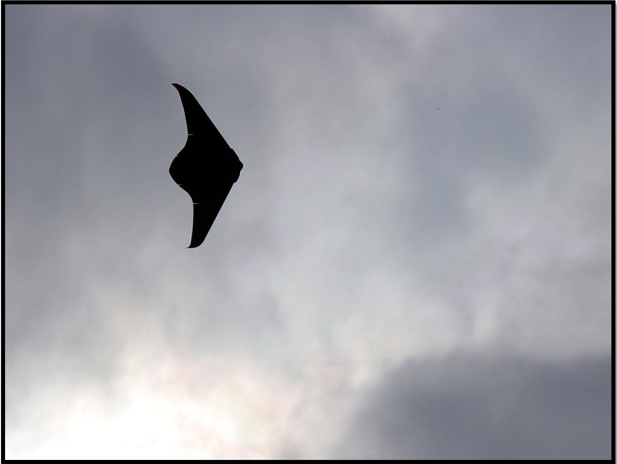
In flight, showing swept planform, raked wingtips and duck tail.
