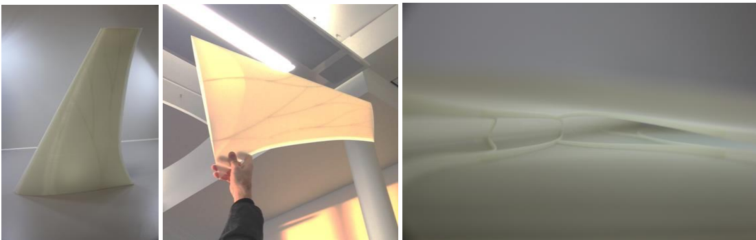
Figure 4 – a) Fully supported wing as printed b) Printed wing c) Internal structure of printed wing
