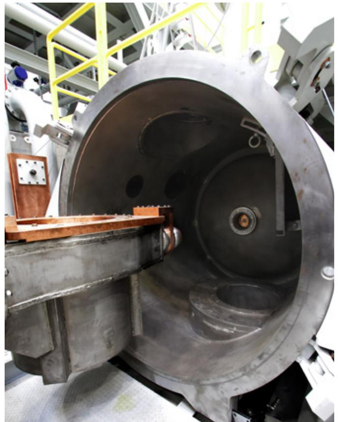
For multi-purpose melting of a range of reactive and other alloys.
