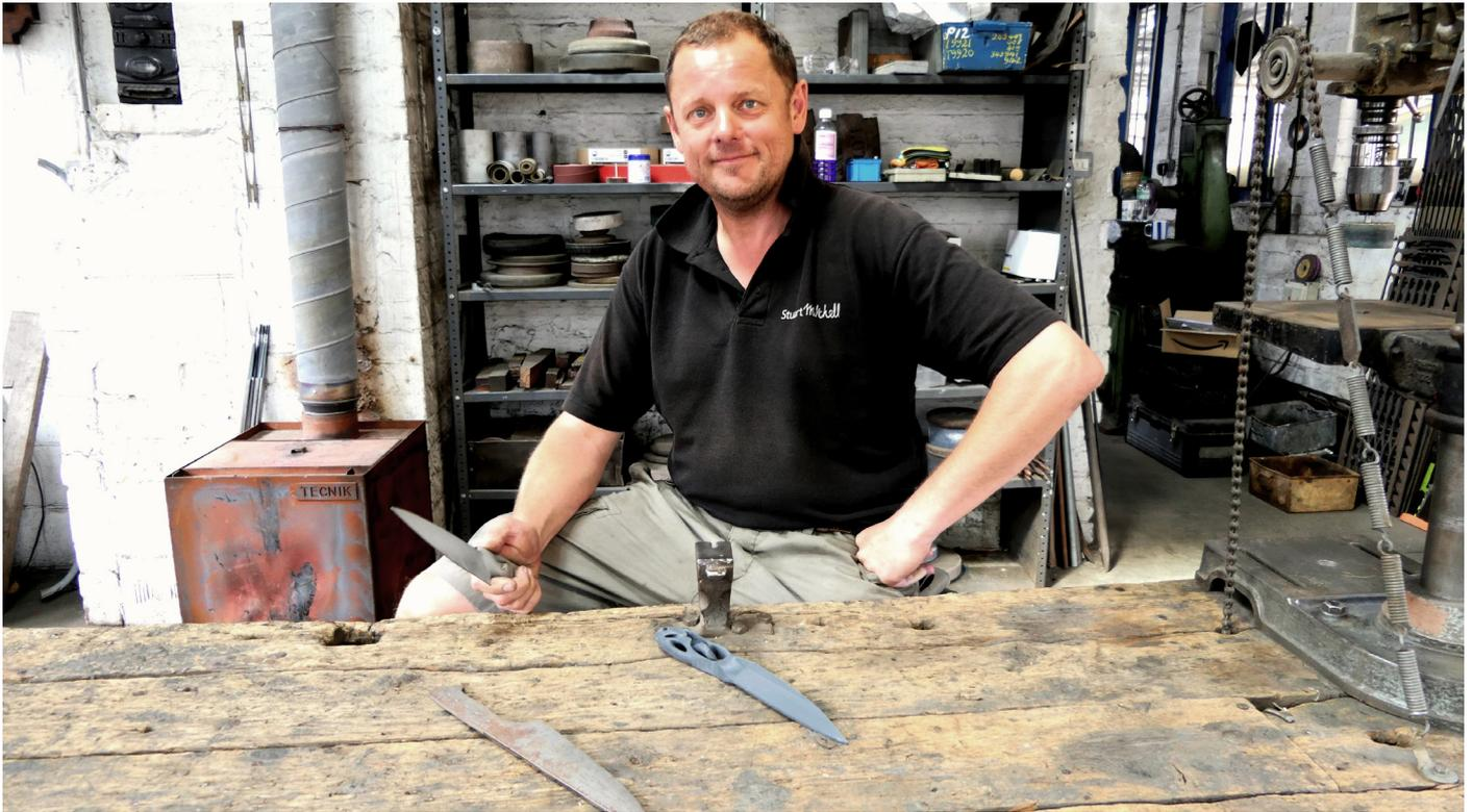
Stuart Mitchell in his Sheffield workshop holding the 3D printed knife blank, with a traditionally made steel blank (left) and the AM prototype (right) on the workshop table.
