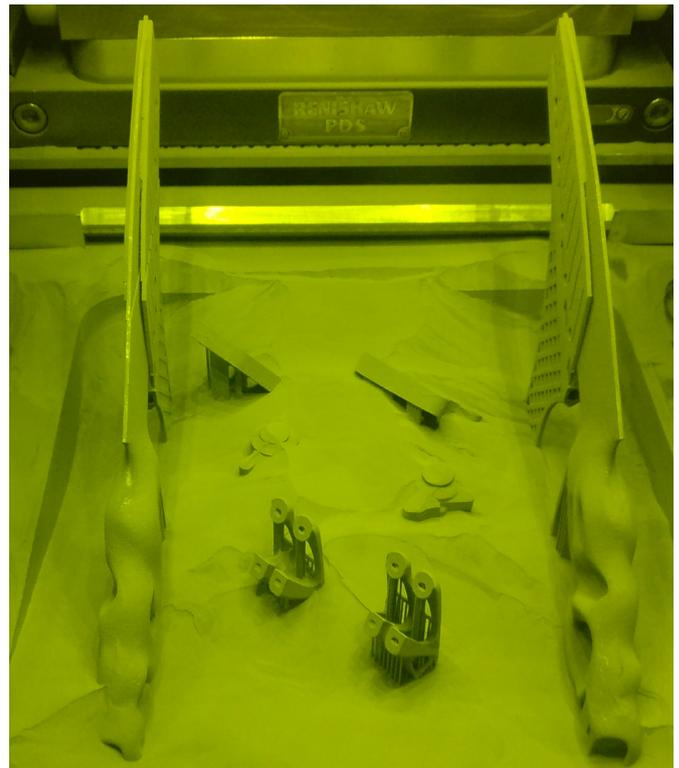
Above shows the knives during the additive manufacturing process and below the end result, complete with the novel support structures and thermal shrouding.
