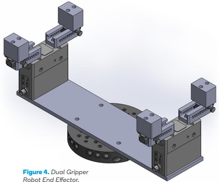
**Figure 4.** Dual Gripper Robot End Effector.
