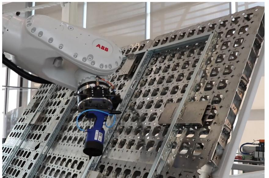
**Figure 5.** Gesipa Rivet Tool.
