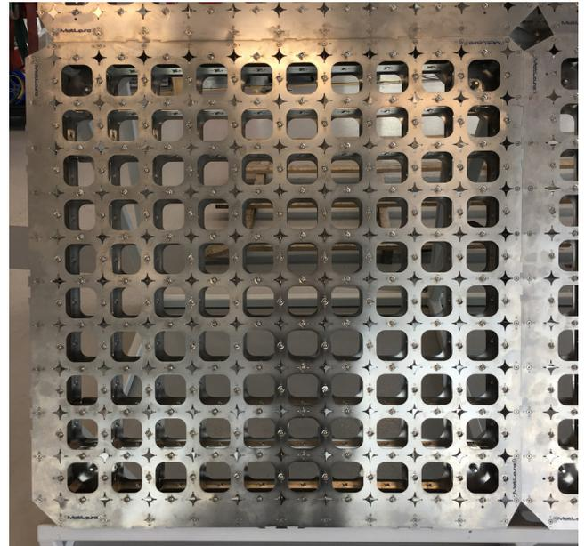
**Figure 2.** MetLase Pegboard Flexible Fixture.
