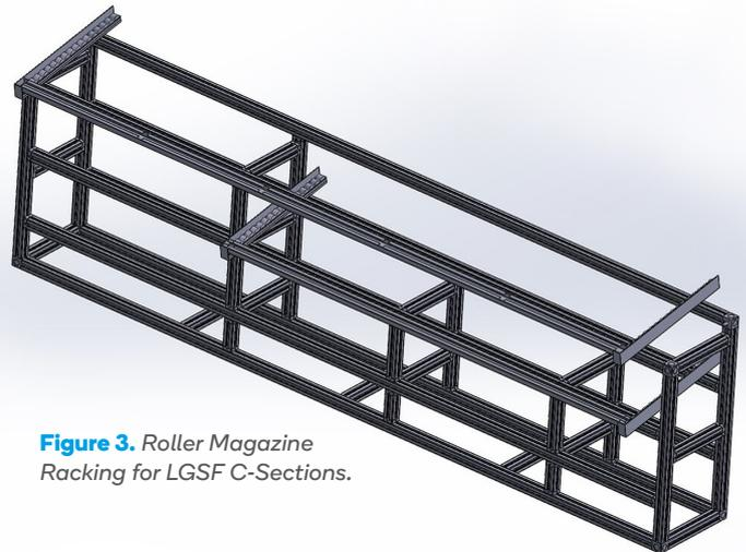
**Figure 3.** Roller Magazine Racking for LGSF C-Sections.
