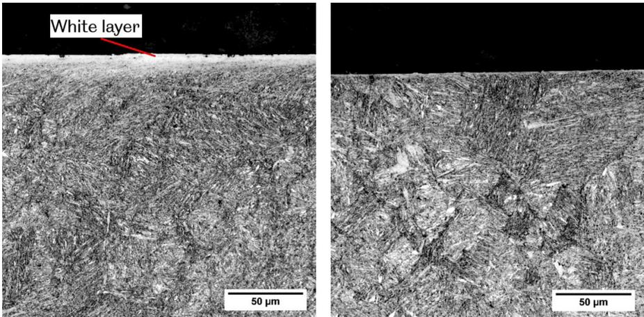
Left: Bad machined surface, created through turning using heavily worn inserts.
