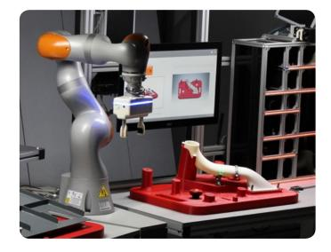
Robotics is already an integral part of BAE Systems' combat aircraft production line which includes a high level of automation, but the integrated sensors that feature in the workstation make it the next step in people safely working directly with robots.
