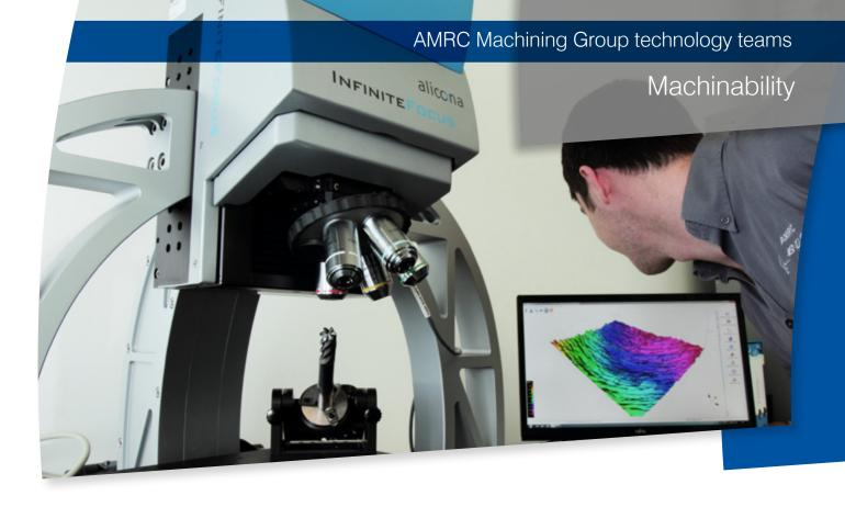
Machinability research underpins the AMRC with Boeing's machining process work, by developing a better understanding of the essential characteristics of high-performance aerospace materials and cutting tools.
