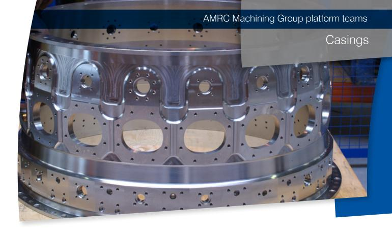
Aeroengine casings have complex geometries and are made from expensive, difficult-to-machine alloys demanded by their increasingly tough operating conditions. Reducing their machining cost while maintaining quality is a critical challenge for many of the AMRC's partners.
