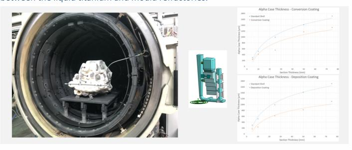
Advances in the investment casting industries has resulted in more developed ceramic moulding systems which yield a more chemically inert surface between the liquid titanium and ceramic mould. These however do still result in a stabilised alpha case layer that requires chemical removal.
