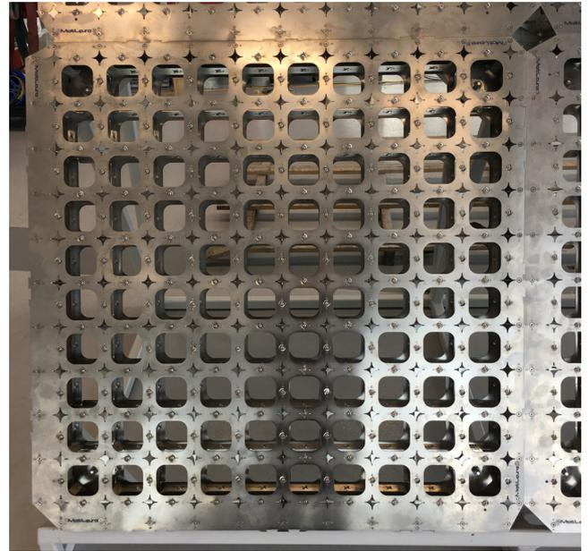
**Figure 2.** MetLase Pegboard Flexible Fixture.
