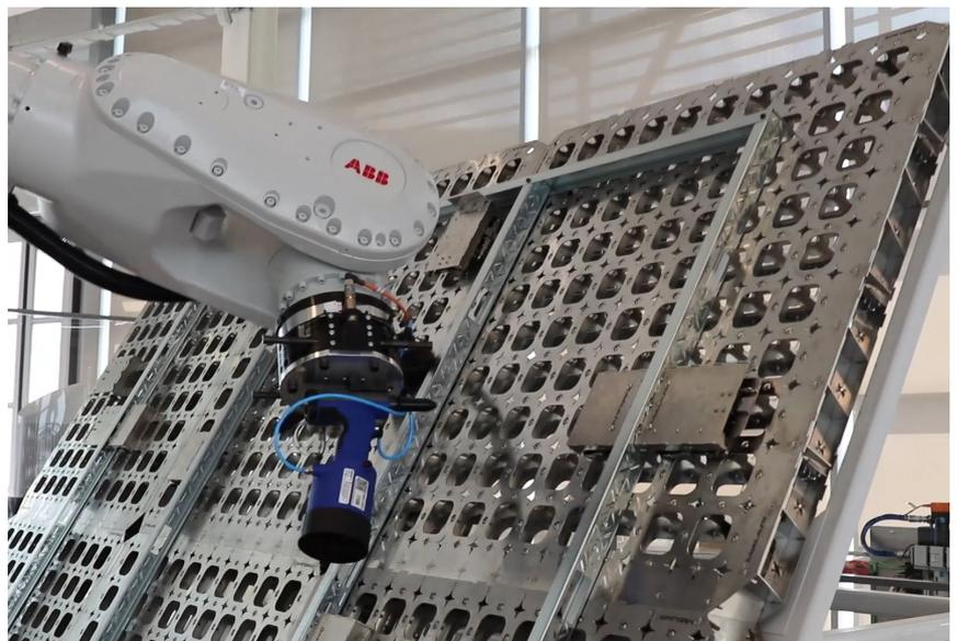
**Figure 5.** Gesipa Rivet Tool.
