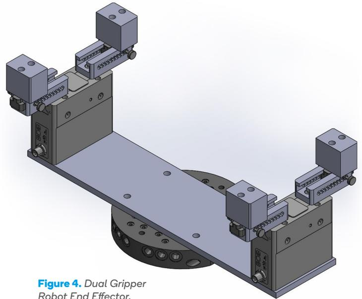
**Figure 4.** Dual Gripper Robot End Effector.
