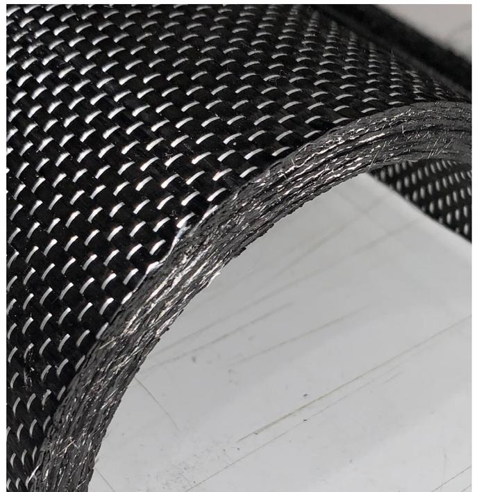
Propeller blade edge showing high quality trimmed surface.
