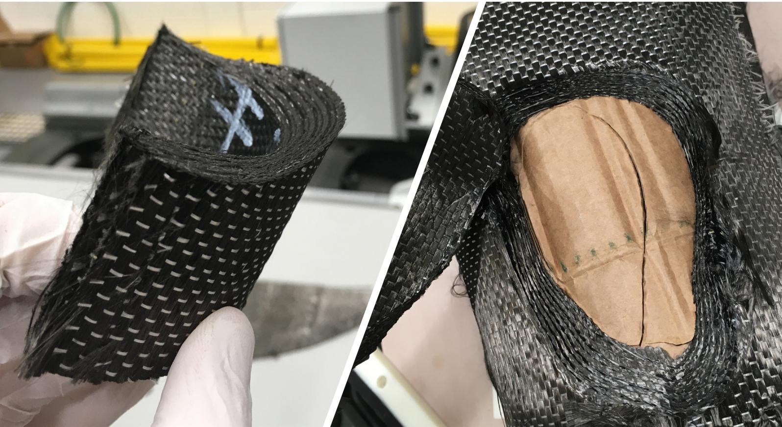
The ultrasonic knife was able to produce chamfered cuts (left) and complex pocket shapes (right) with high accuracy.
