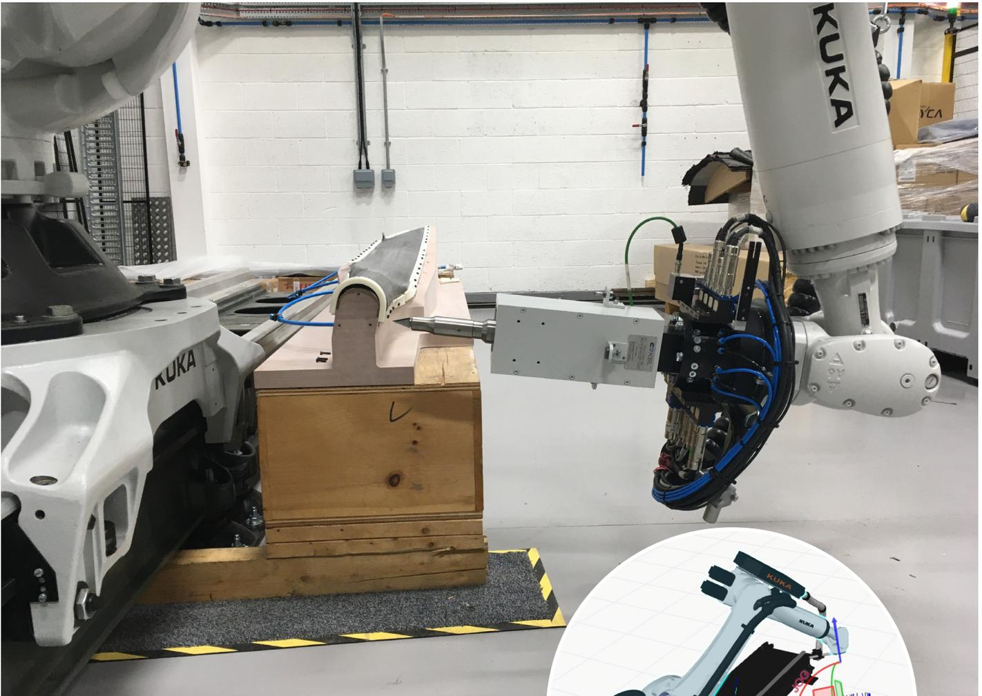
The AMRC's KSL robot cell with ultrasonic knife attachment. KukaSim (inset) was used to work out the ideal position for the tool for the optimum cutting path.
