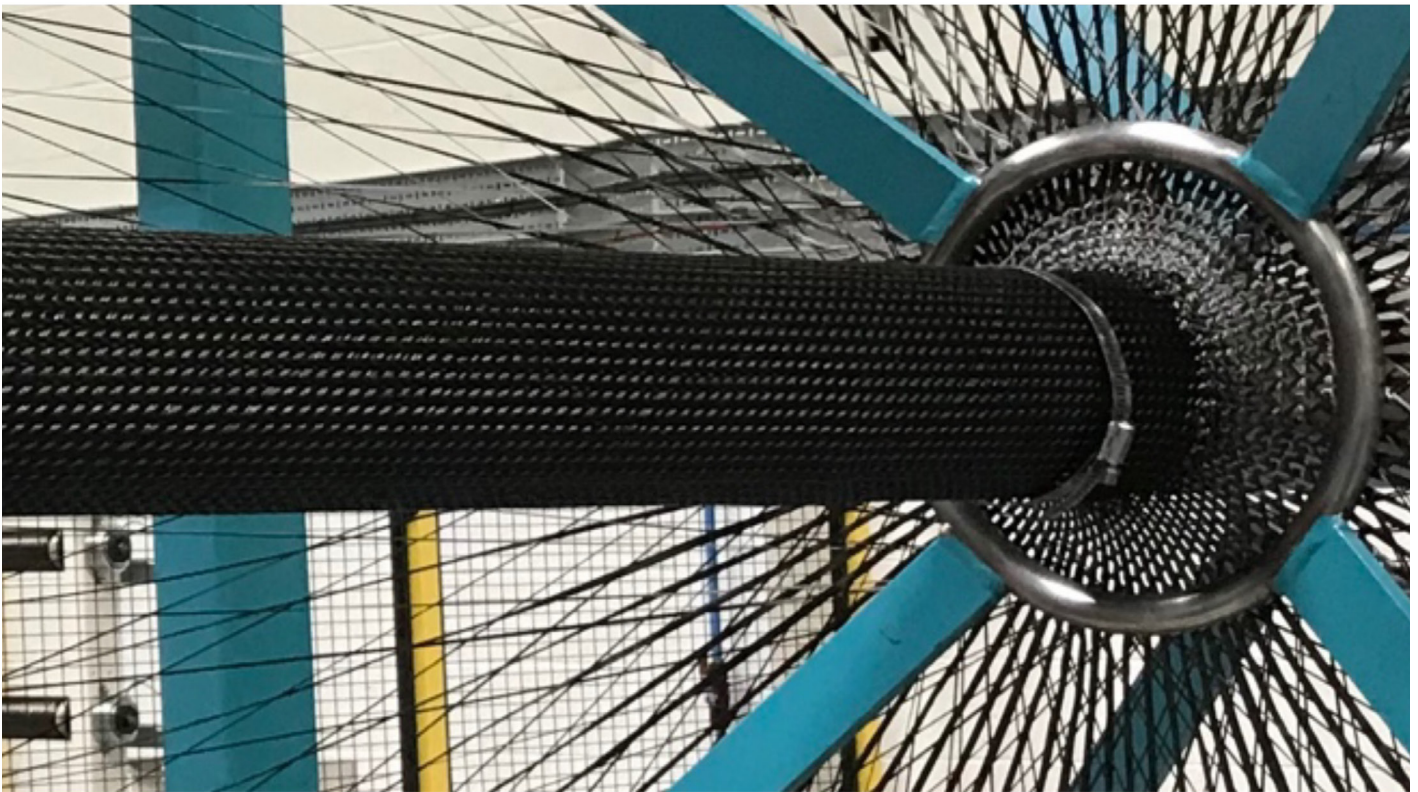
Development trials were conducted on tubular mandrels to optimise the machine set-up to produce the desired complex braid structure.
