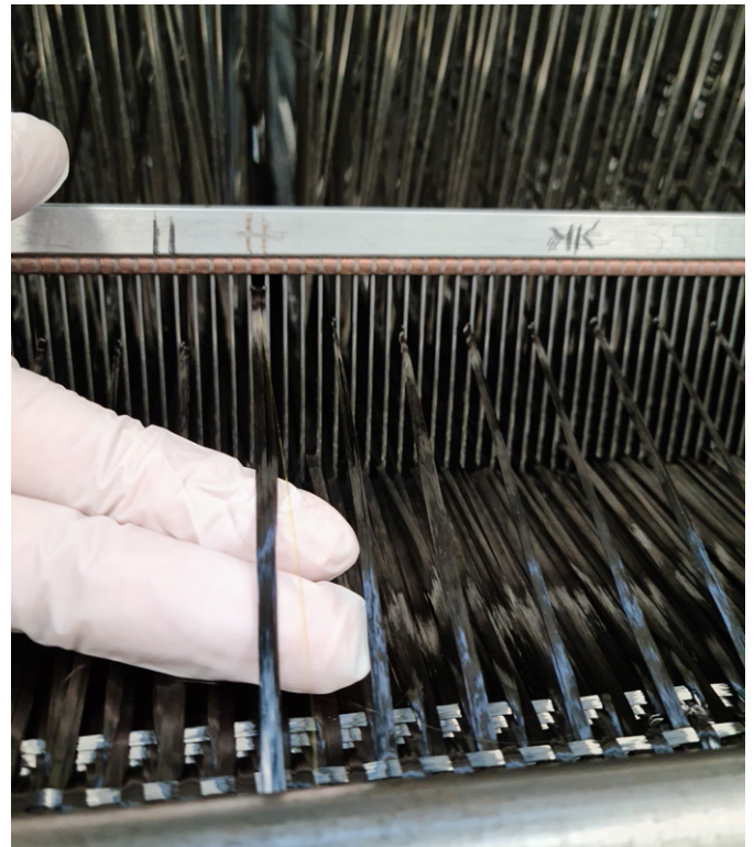
Fibre optic sensors were inserted with a carbon fibre in the warp direction.
