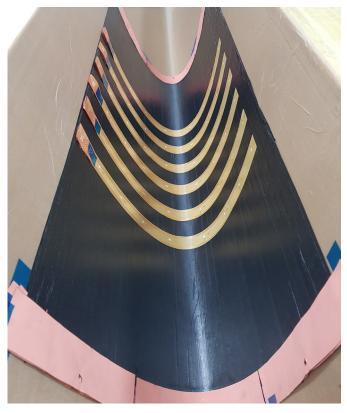
Final demonstrator during manufacturing, showing modular selfsensing PCBs being laid up equidistant apart, to provide high density of electrodes to ensure the system is sensitive to damage.
