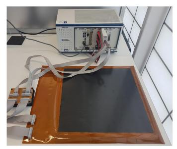
The initial test setup, showing the resistance data acquisition system and the flexible PCB embedded into the composite panel.
