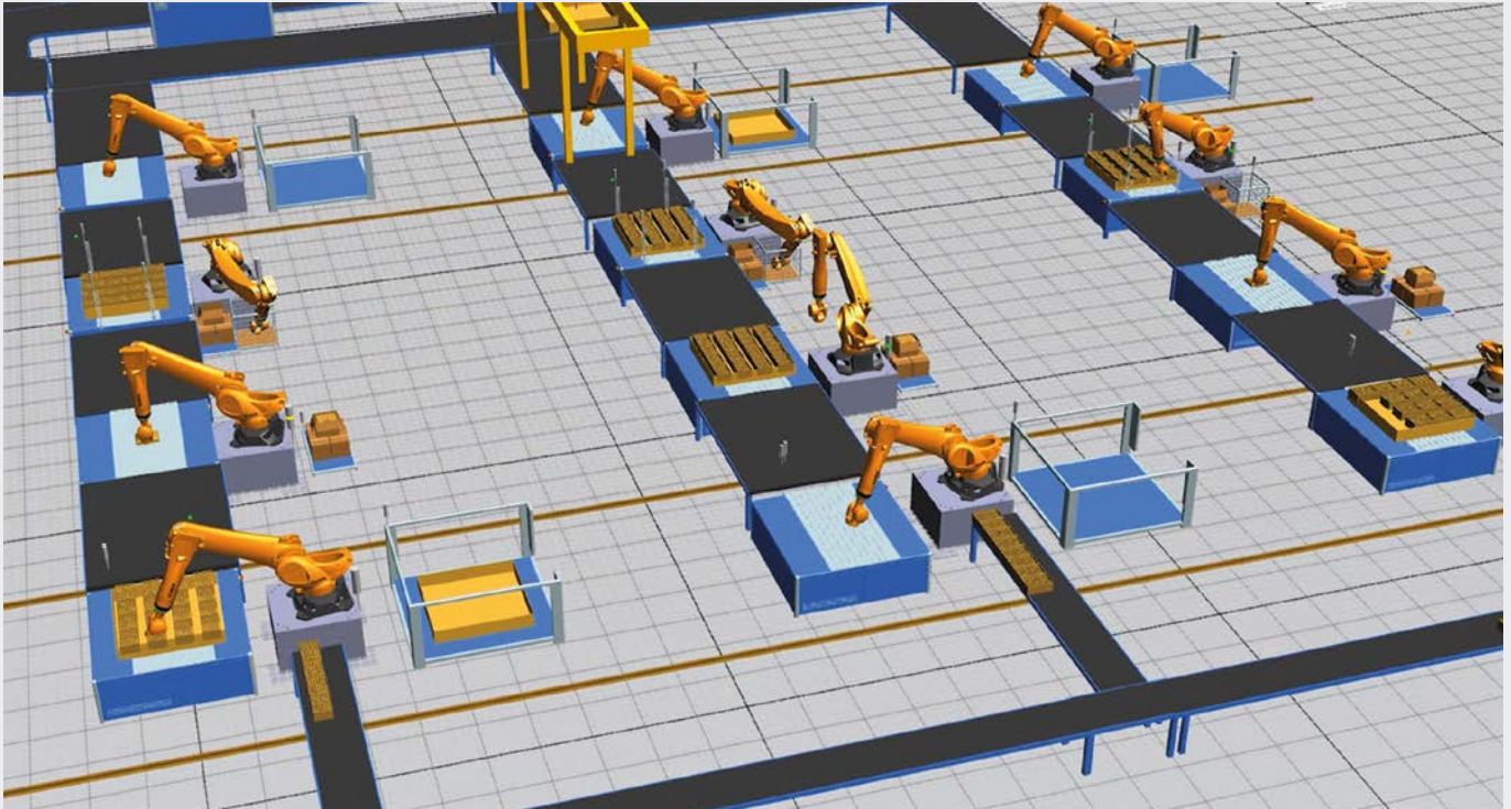
The model integrates key process elements such as automated conveyor systems and robotic arms to demonstrate material flow, machine utilisation and process interactions.
