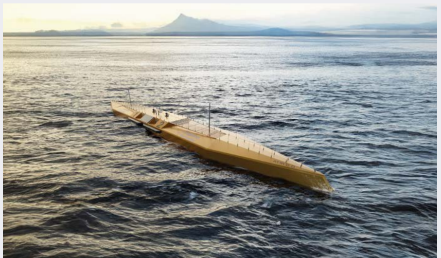
ATIR 2.0, Magallanes' world's first future tidal energy converter.
