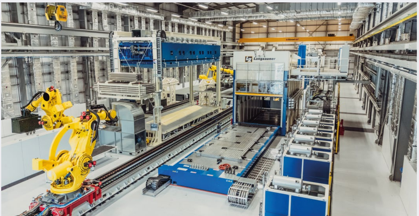
Inside COMPASS: Housing giant 1,700kg-capacity industrial robots and the world’s largest-of-its-kind RTM press – delivering the future of high-rate manufacturing at speed, scale and precision.
