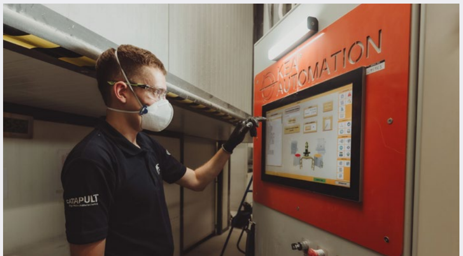
Jack Naylor interacting with the automated shelling system to test mould production with iMOLD sensor data tracking.
