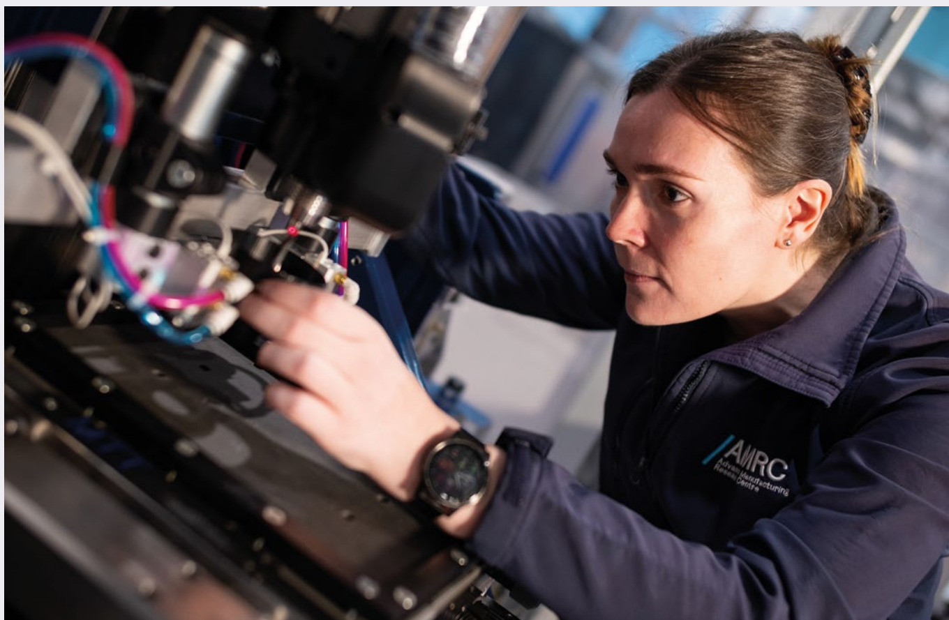
Innovation fellow Erica Smith sensorising the new AMRC Cymru drilling and fastening cell.
