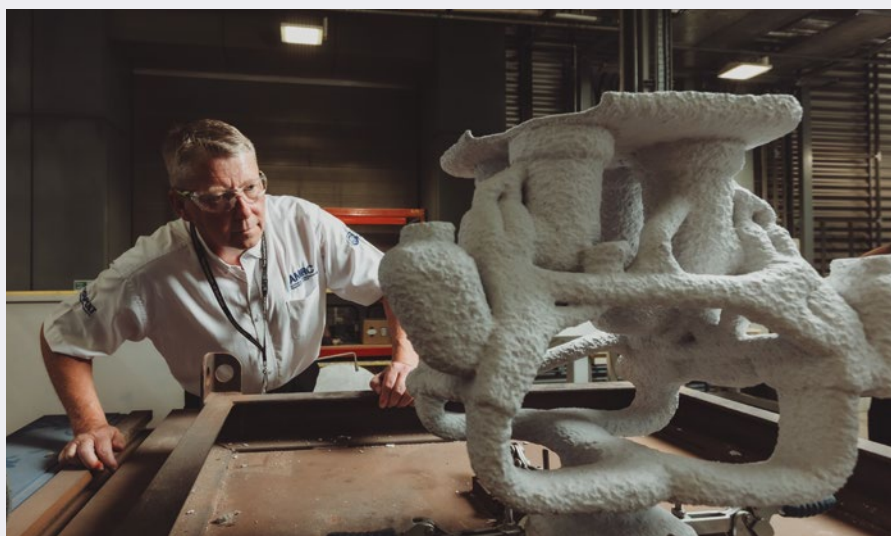
Matt Cawood pictured alongside the counter-gravity platform that was used to produce a single aircraft casting, consolidated from a nine-part assembly.
