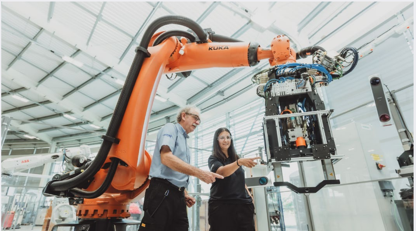
Phil Yates, technical fellow and Lucy Mello, machine integration engineer for automation, looking at the end effector of the Spirit Views robot cell, which is being used to test machine learning (AI) methods to improve robot accuracy.
