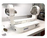
Smart Fixture with integral sensors and weigh scales
